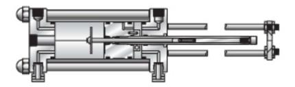
The pistons, end caps, indicating rods, mixers, tie rods, and nuts are all fashioned from 316 stainless steel. The cylinder is also constructed of 316 SS. The stainless steel construction of our constant pressure sample cylinders gives them excellent resistance to corrosion and exceptional longevity.
